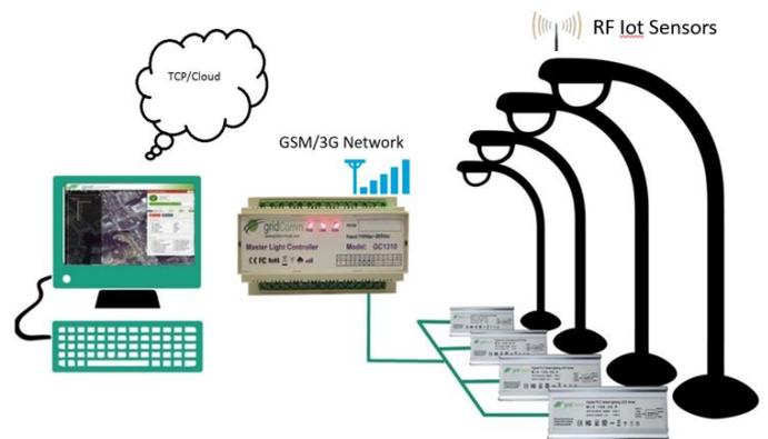
**Figure 2- Smart Street Light Control System**
