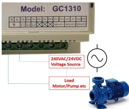
Figure 6- Dry Contact Relay Control
