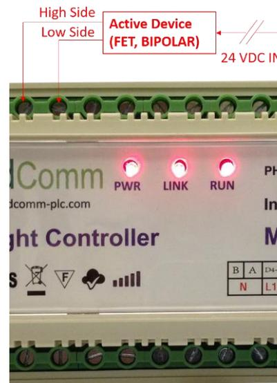
Figure 4- Digital Inputs of GC1310
