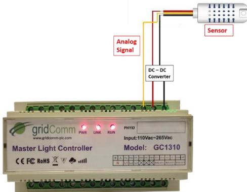
Figure 5- Analog Inputs of GC1310
